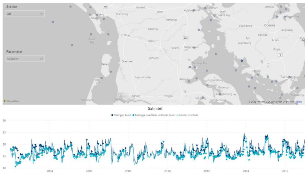
Figure 3-18: Example of comparison between model results and data (Station in Helnæs Bay, salinity), (DHI 2022) RBMP (dhigroup.com)
