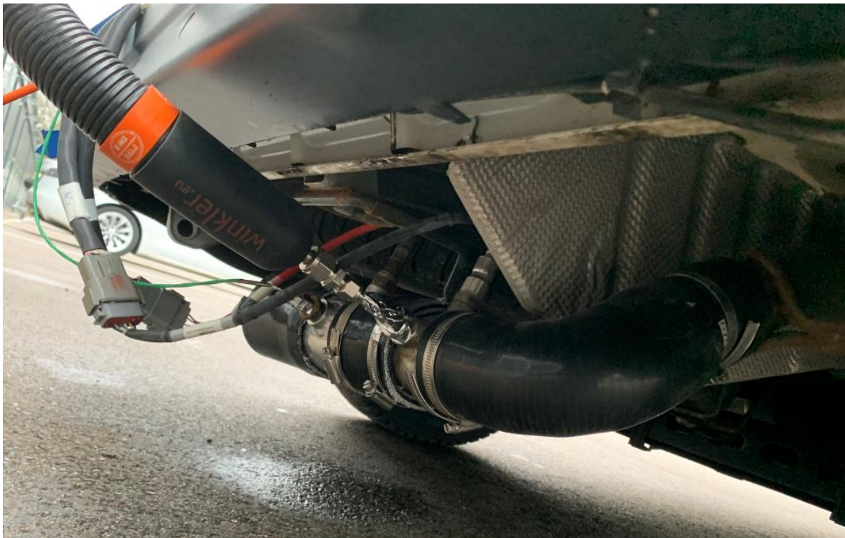
Figure 28. Test probe mounted in exhaust pipe. The heated line is for particle measurement and the sensors for NO x , CO, CO 2 , O 2 , lambda.
