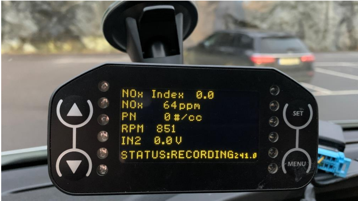
Figure 27. Test set-up inside the cabin. From this screen the logging were start and stopped. It is also possible for the driver do follow the trends etc. There are 5 different pages on the screen
