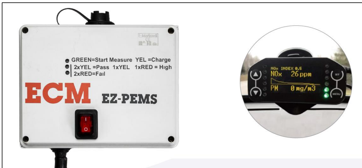
Figure 6. The EZ-PEMS system. To the left the main unit to which the sensor is connected. To the right is the display where real time data can be viewed and buttons to control start and stop of the tests. After stop of a test the data is uploaded to the cloud and reports are automatic generated.
