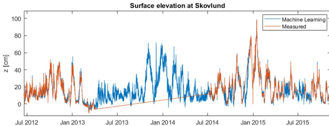
Figure 4.6 Gap in water level measurement at Skovlund, filled with machine learning regression.
