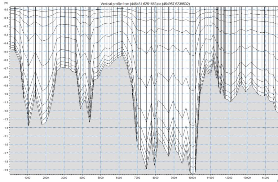
Figure 4.3 Vertical model mesh of the Nissum Fjord model in transect from North-West to South-East, with 10 sigma-layers refined towards the surface and fjord bed.
