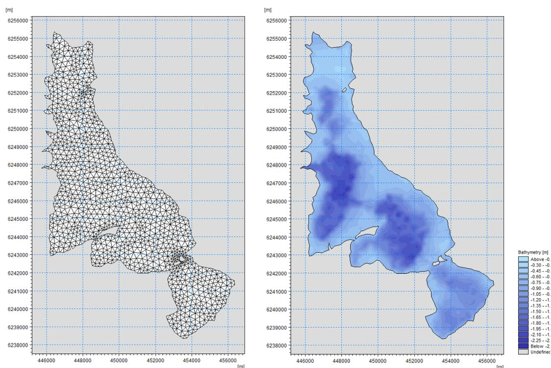
Figure 4.1 (Left) horizontal mesh and (right) bathymetry of the Nissum Fjord model. Map projection ETRS-1989-UTM-32 and vertical datum DVR90.
