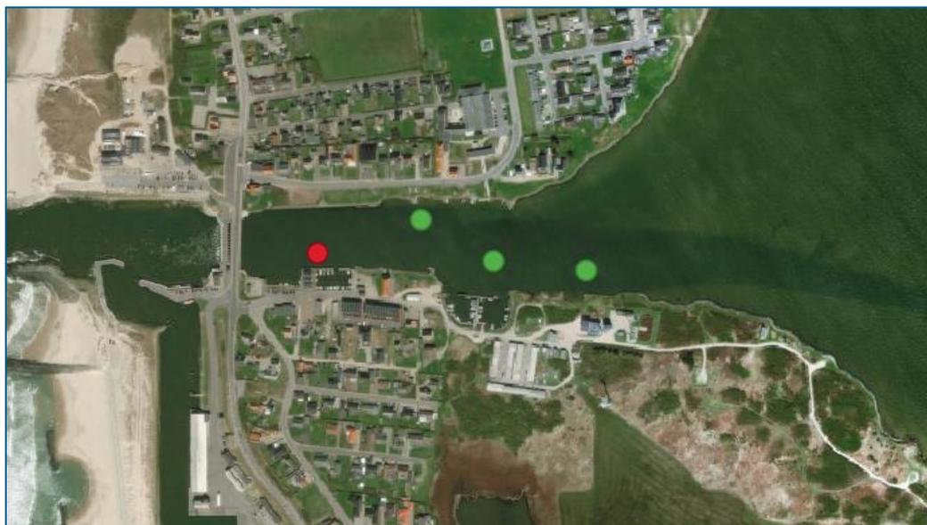
Figure 4.7 Location of sluice sources in Thorsminde. The red point represents five outflow sources, which were placed in sigma-layers 4-8. Each green point represents one or two inflow sources which were placed in the sigma-layers 1-2.
