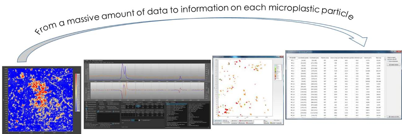
Figure 6. From an  $\mu$ FTIR map holding millions of individual spectra to identified microplastic particles, including their size, polymer type, shape and mass ([www.simple-plastics.eu](http://www.simple-plastics.eu))
