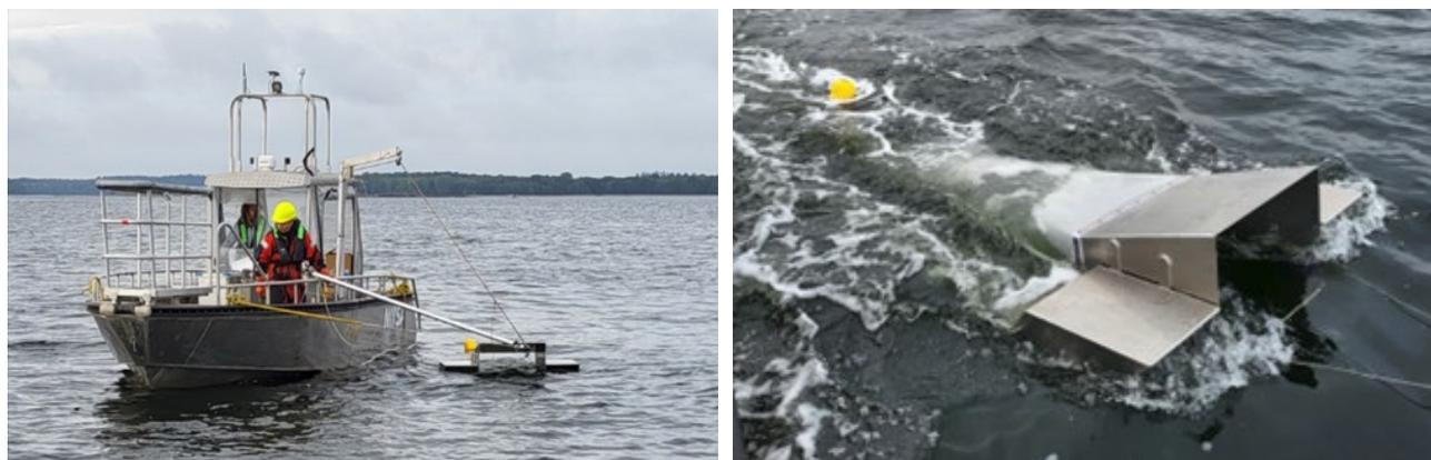
**Figure 3.** Sampling microplastic with a 70 cm wide manta trawl alongside a small vessel in Danish coastal waters in 2022.
