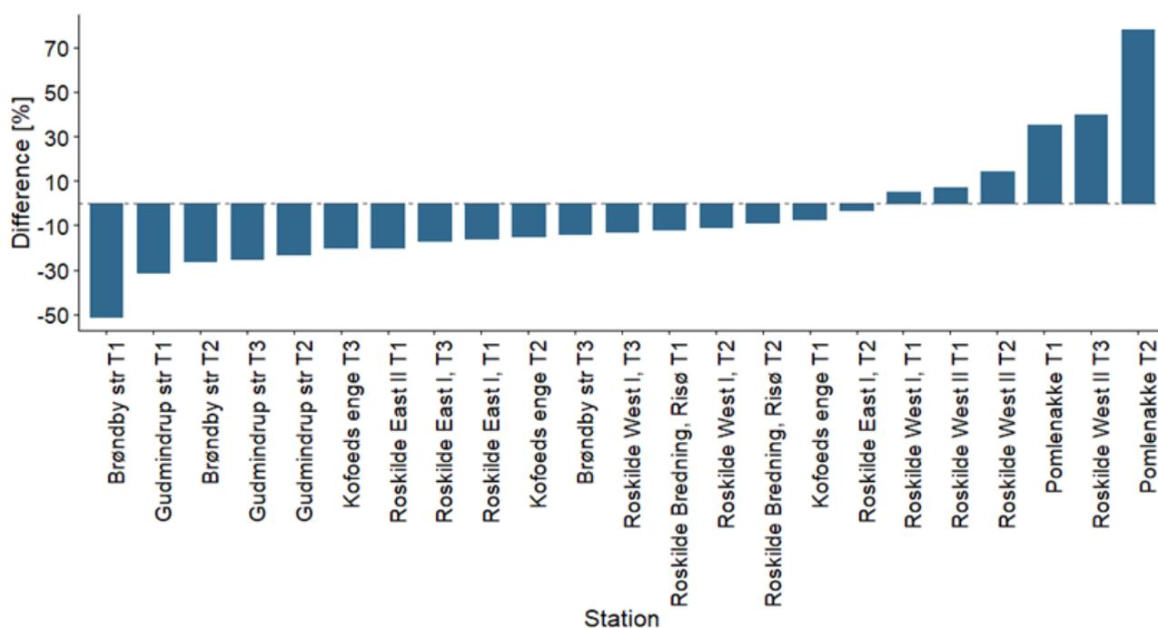
**Figure 13.** The difference between the sampled volume calculated from the flowmeter readings and based on the travelled distance determined by GPS coordinates.
